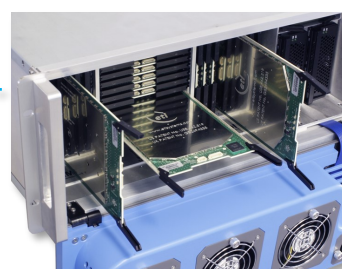
Hot-swap, input matrix cards (IMC), middle matrix cards (MMC) and output matrix cards (OMC)
