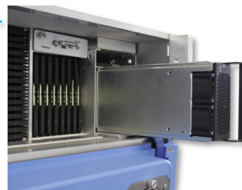
Hot-swap, dual redundant power supplies
