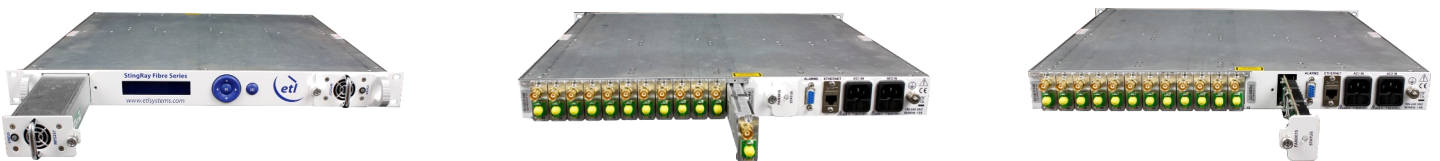
Indoor chassis showing hot-swap power supply modules, fibre modules & fans
