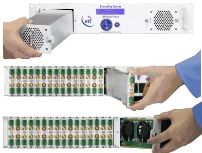
Indoor chassis showing hot-swap power supply modules, fibre modules and fans
