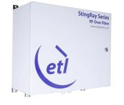
The StingRay RF over Fibre Outdoor unit (ODU) is a robust weatherproof (IP65 rated) enclosure which has been designed to be wall or post mounted close to the antenna. It can accommodate up to 10 Transmit or Receive 200 series StingRay Fibre modules.
