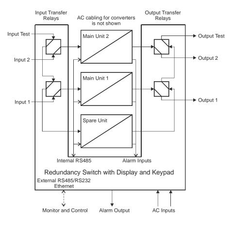
2:1 Redundancy Switch System with RSCC-2
