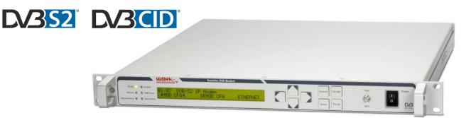
WORK Microwave's high-speed DVB-S2 IP modem SK-IP provides operators with a platform for transferring IP/Ethernet data over DVB-S2 satellite connections. Ethernet frames and IP packets are encapsulated directly within DVB-S2 baseband frames, resulting in low encapsulation overhead.
