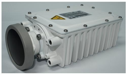
The Global Skyware Limited XRF transceiver is the result of applying the industry's cutting edge Ka-Band VSAT engineering techniques and production methods to result in our lightest, most compact and affordable design to date. The ruggedised IP-67 sealed enclosure integrates a BUC, LNB, field-configurable circular polariser, and TRF guaranteeing consistent communications performance. The XRF transceiver additionally includes audible pointing assistance to simplify installation.
